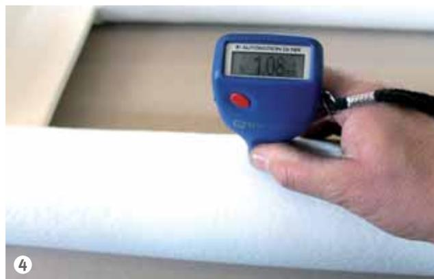
Figure 4: Coating thickness measurement with Automation Dr: Nix thickness gauge, distributed in Italy by Tecno Supply.
